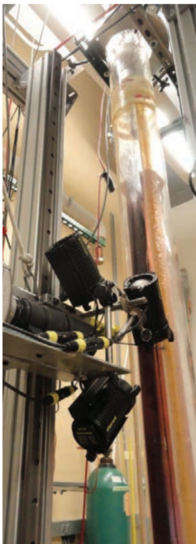
Jaeger's experimental setup includes a camera that drops in near free fall with the charged grains, capturing their interactions as they drop through an airless tube.
