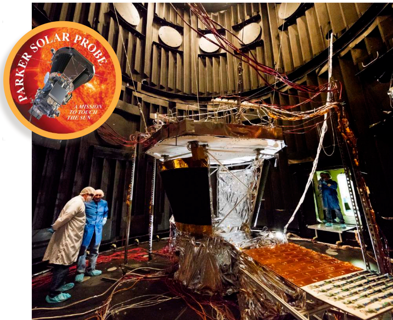
The Parker Solar Probe will draw power from its solar arrays, so protecting them from the extreme environment near the sun is vital to the mission's success. Here, one element of the solar array cooling system undergoes testing at NASA's Goddard Space Flight Center in February.
