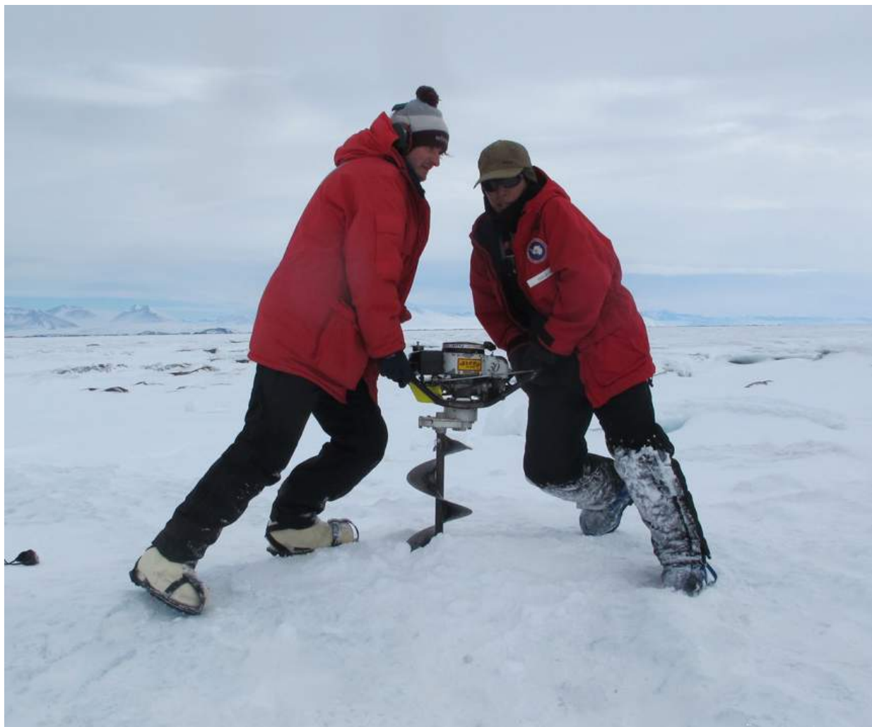
Physical Sciences Division graduate student Grant MacDonald and a National Science Foundation collaborator install a seismometer in an ice shelf to detect tremors associated with fractures and meltwater movement.
