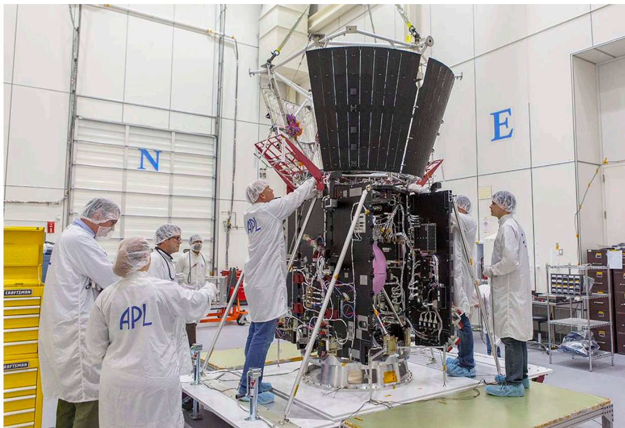
In April 2017 engineers at the Johns Hopkins University Applied Physics Laboratory installed key components of the Parker Solar Probe's cooling system. The spacecraft will be protected by a 4.5-inch-thick, 8-foot-wide carbon-composite heat shield designed to withstand the blistering temperatures it will face on its journey to the sun.
